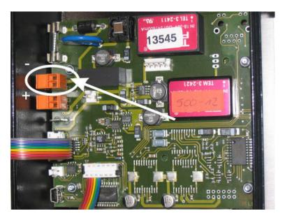
The power supply connector is one of the orange connectors on the main PCB, the one close to the fuse. Connect the (-) cable to the connector close to the fuse and the (+) cable to the other pin of the connector. The connectors may be pulled off the PCB for easier access. Please note that the power connectors may be hidden below the AUX-PCB, if you order that as an option.
