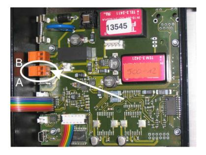
Please connect the terminal labelled "A" with the same label on the transmitter side. The "A" terminal may also be labelled "+" or "1". Connect the "B"-terminal to the connector with the label "B", "-" or "2" on the transmitter side.
